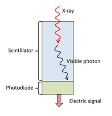
There is a solid scintillator layer that converts the x-rays into visible light photons. The photodiode then converts the photon input into an electrical signal.
