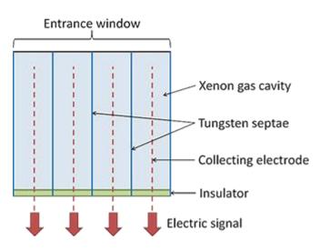
The detector array is a single vessel filled with gases of a high atomic number (Krypton / Xenon) and subdivided into separate detectors by tungsten septate.
